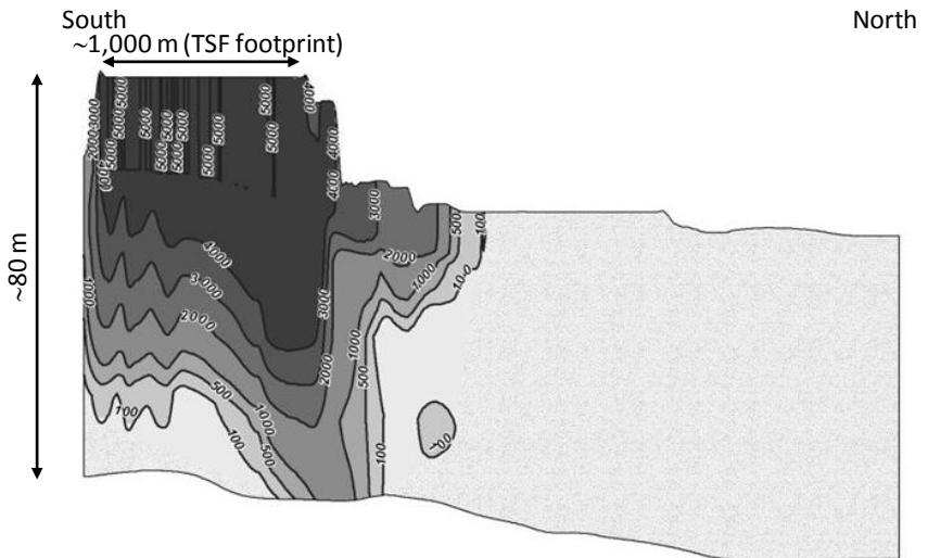
**Figure 3** Predicted sulfate concentrations (mg/L) (cross-section view through centre of TSF)
