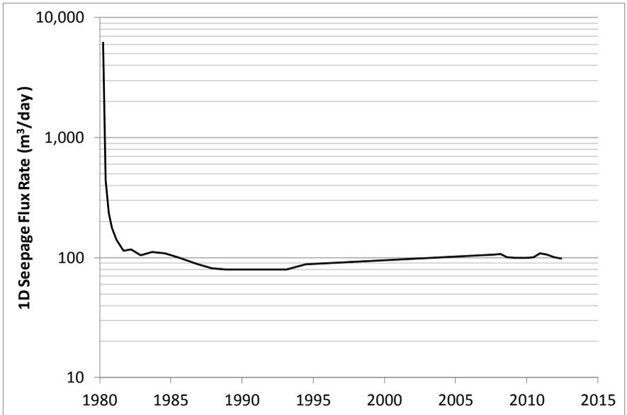
**Figure 2** Estimated total seepage flux from the base of the TSF ("central estimate")
