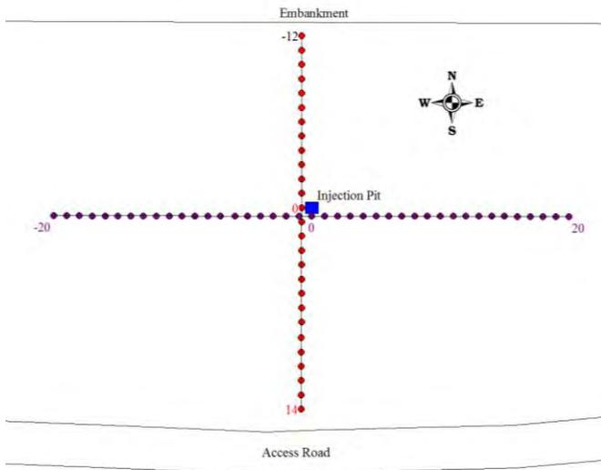
**Figure 4** Survey geometry employed during the ERT investigations.
