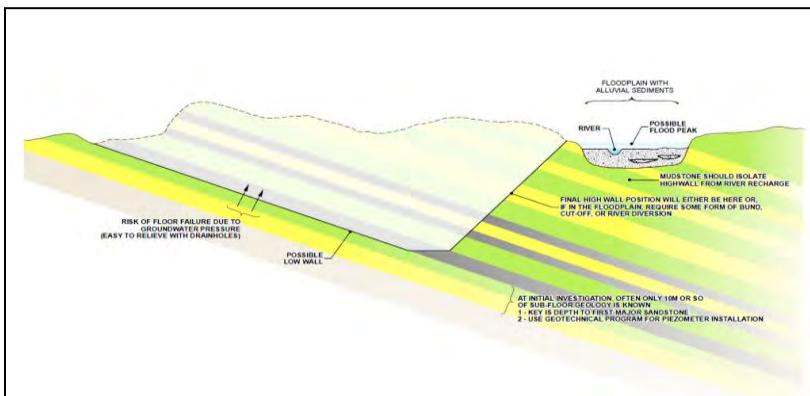
**Figure 2:** Schematic diagram of mine with surface water adjacent to high wall perimeter
