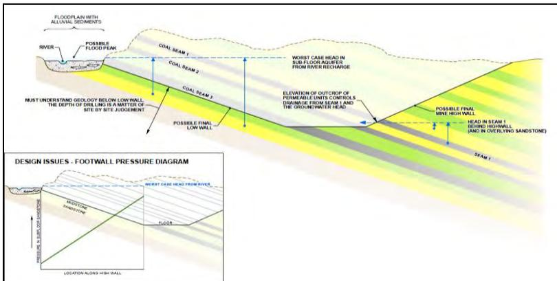
**Figure 1:** Schematic diagram of mine with surface water adjacent to low wall perimeter
