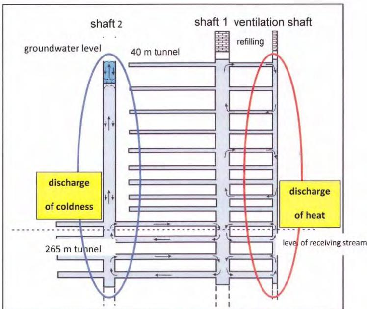
**Figure 1** Schematic diagram of the mine and its potential for a sustainably exploited geothermal storage reservoir
