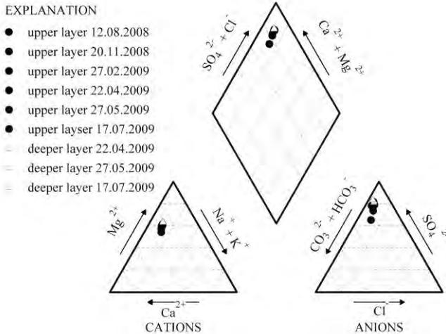
**Figure 2** Piper diagram of mine water shaft 2
