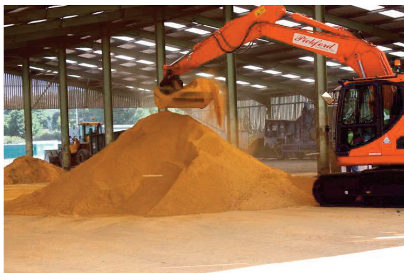
Fig. 1. Mine water treatment HFO being blended with iron(II) sulphate at a UK location
