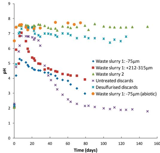
**Fig. 4** Batch biokinetic test results for wastes from coal processing
