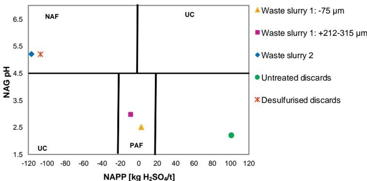
**Fig. 3** Static ARD classification plot for the coal processing wastes (NAF: non-acid forming, UC: uncertain, PAF: potentially acid forming and AF: acid forming)
