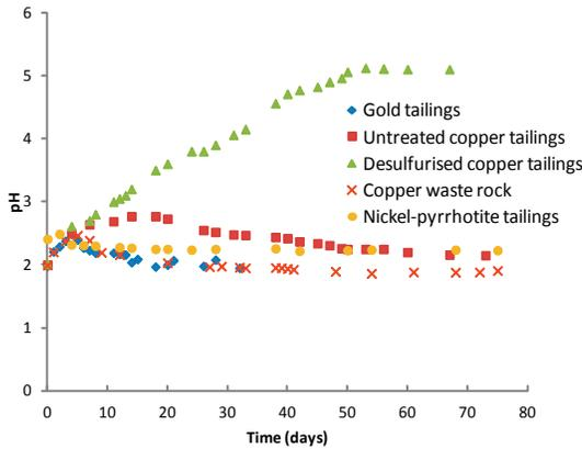
**Fig. 2** Batch biokinetic test results for wastes from the processing of hard-rock ores
