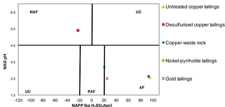
**Fig. 1** Static ARD classification plot for the wastes from hard-rock ore processing (NAF: non-acid forming, UC: uncertain, PAF: potentially acid forming and AF: acid forming)
