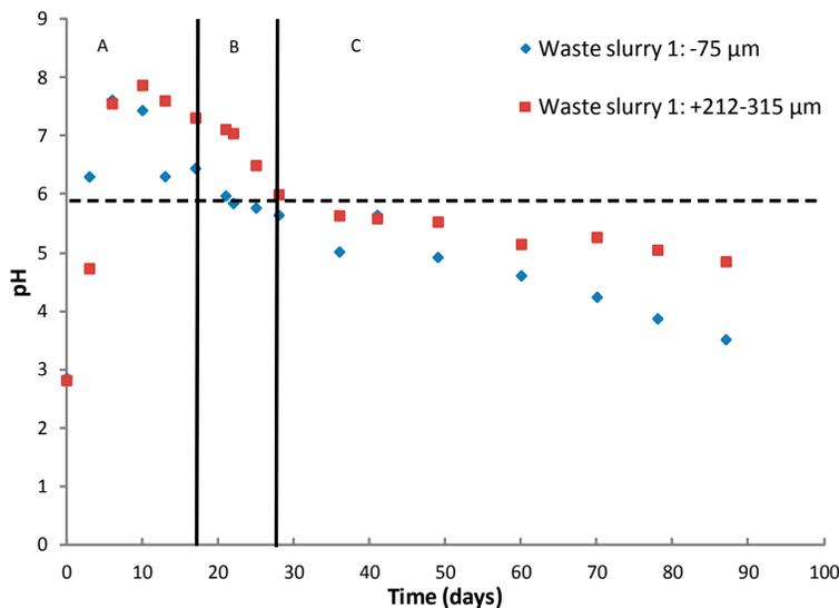
**Fig. 5** Dynamic biokinetic test results for wastes from coal processing at circum-neutral pH conditions (where A, B and C correspond to supernatant replacement intervals of 3, 8 and 14 days respectively)
