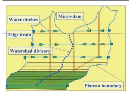
**Fig. 7** Schematic sketch of the location of micro-dams in drainage channels.
