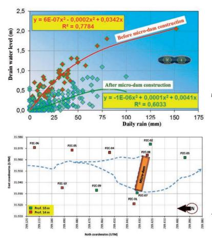
**Fig. 8** Height of water next to the drain before and after the construction of the impoundments.
