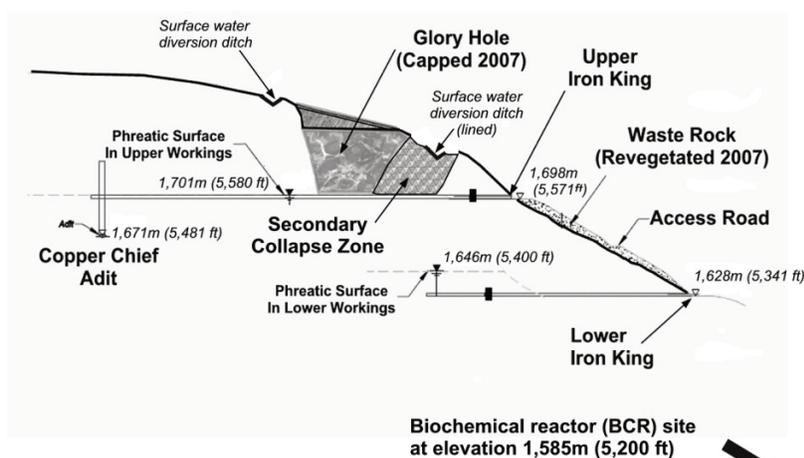
**Fig. 1** Underground mine schematic cross section
