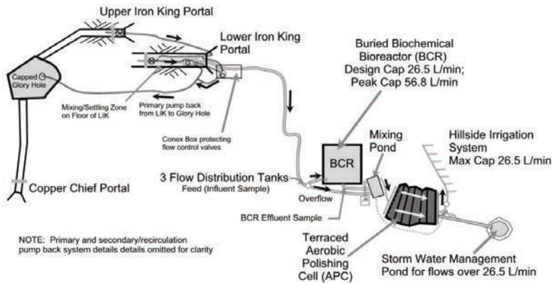
Fig. 4 Passive treatment system (PTS) schematic
