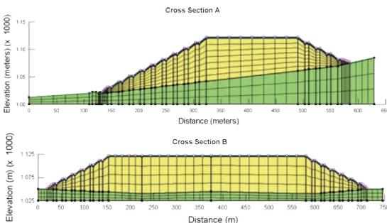
**Fig. 1** Facility cross-sections and model construction.
