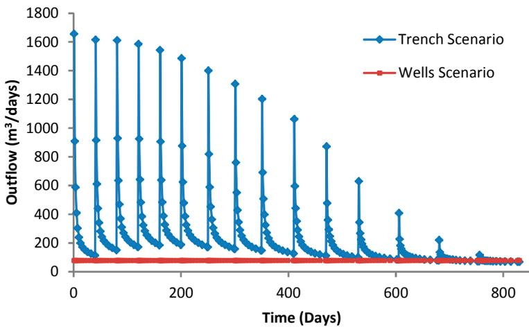
**Fig. 4** Estimated dewatering rates for two methods of dewatering: trenches and pumping wells
