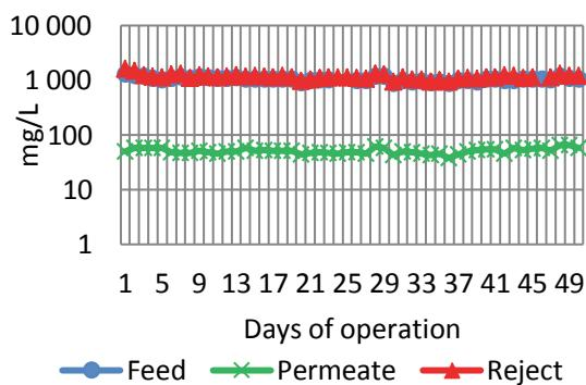
**Fig 7** Sulfate feed, permeate and reject
