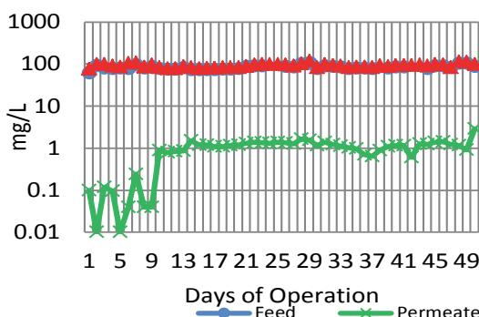
**Fig 6** Manganese feed, permeate and reject
