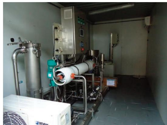
**Fig. 5** Nanofiltration System
