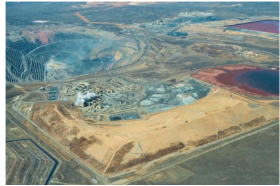
Fig. 2 Freshly reclaimed AA Leach Pad showing drainage network on the cover surface (looking northwest).
