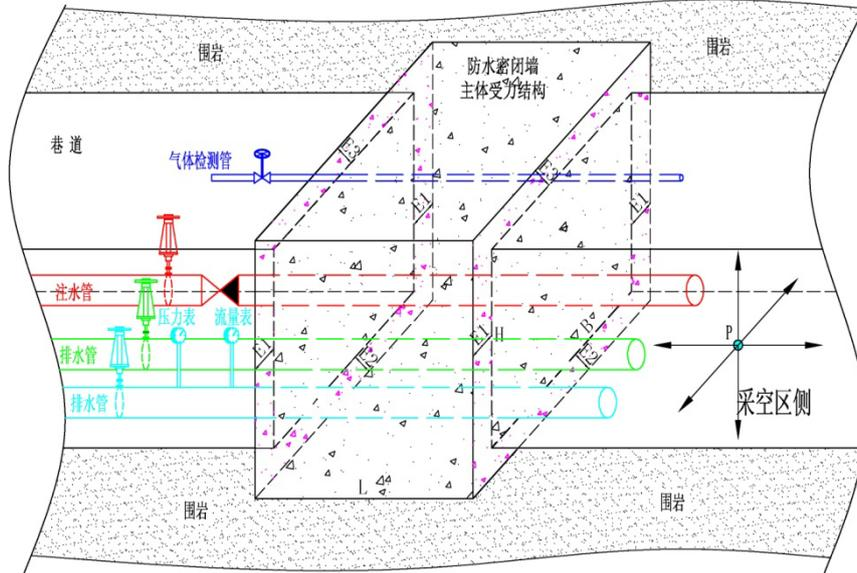
Fig. 2 Structural Diagram of Waterproof Sealing Wall
