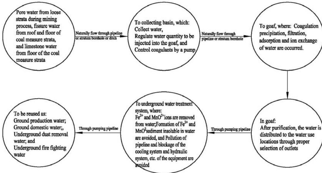
Fig. 1 Process flow diagram for mine water reuse in underground goaf
