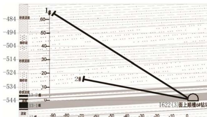
*Fig.1 Profile of electric method detection borehole layout section*
