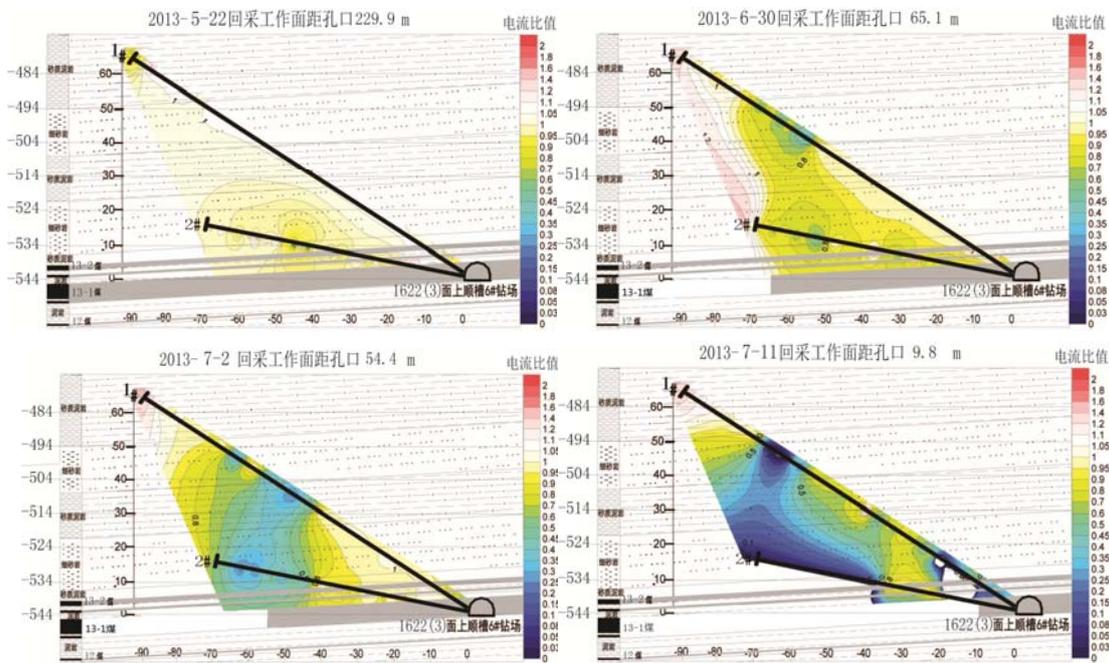
*Fig.2 Distributing map of the strata distribution of current ratio in rock of collapsing belts*
