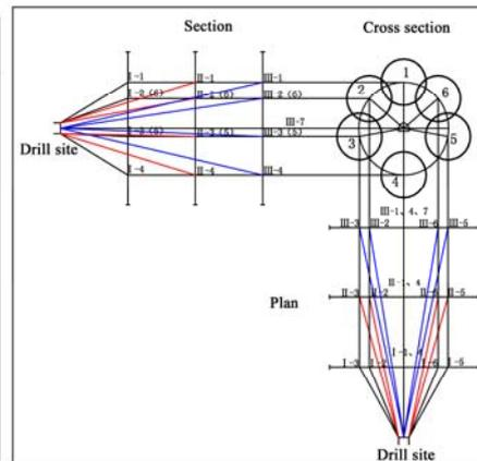
*Fig. 2* plan, section & cross section of drill holes for curtain grouting
