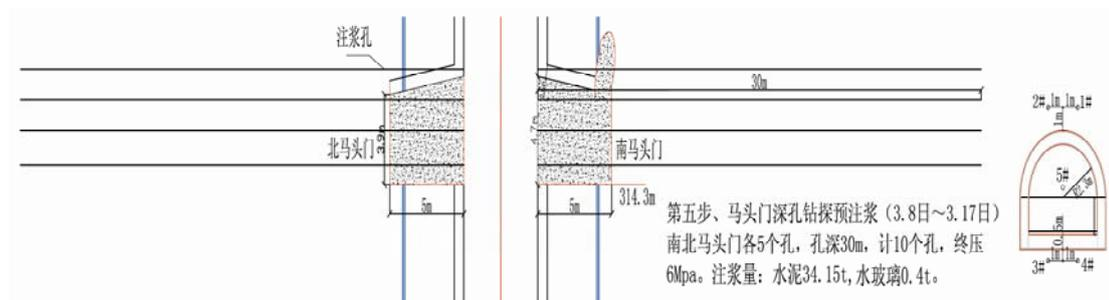
Fig. 5 Layout diagram of advanced exploration and preliminary grouting holes of ingate
