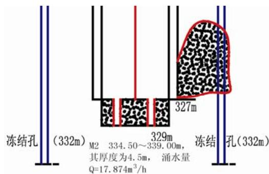
Fig. 1 Layout diagram of the grouting pad and lodgement at the bottom hole
