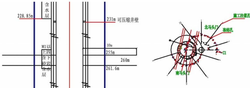
Fig. 3 Layout diagram of grouting holes in the sandstone formation between M1 and the "fourth aquifer"
