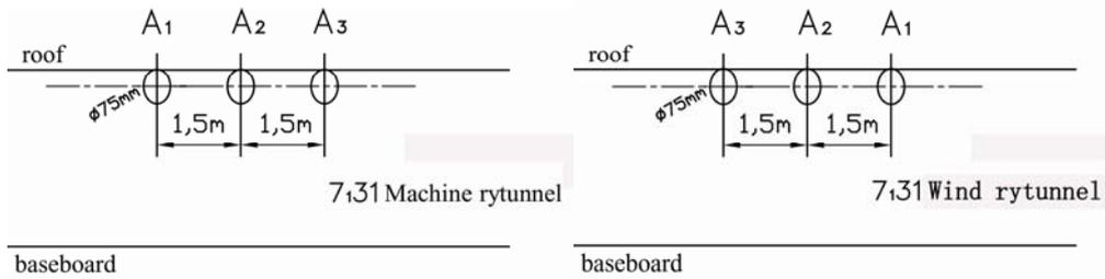
Fig. 1 Layout chart of presplitting holes
