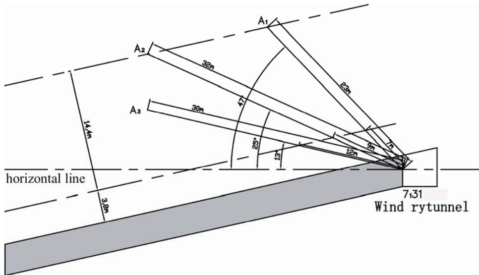
Fig. 2 Designed layout chart of presplitting holes
