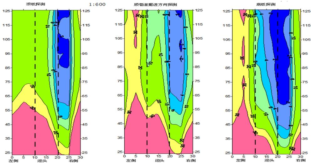
Fig.3 Apparent resistivity abnormal areas in the working face of roadway 720
