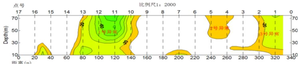
Fig.2 Apparent resistivity abnormal areas in the wall of belt entry II51
