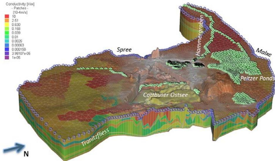
Fig. 2 FEFLOW model with applied conductivities and boundary conditions
