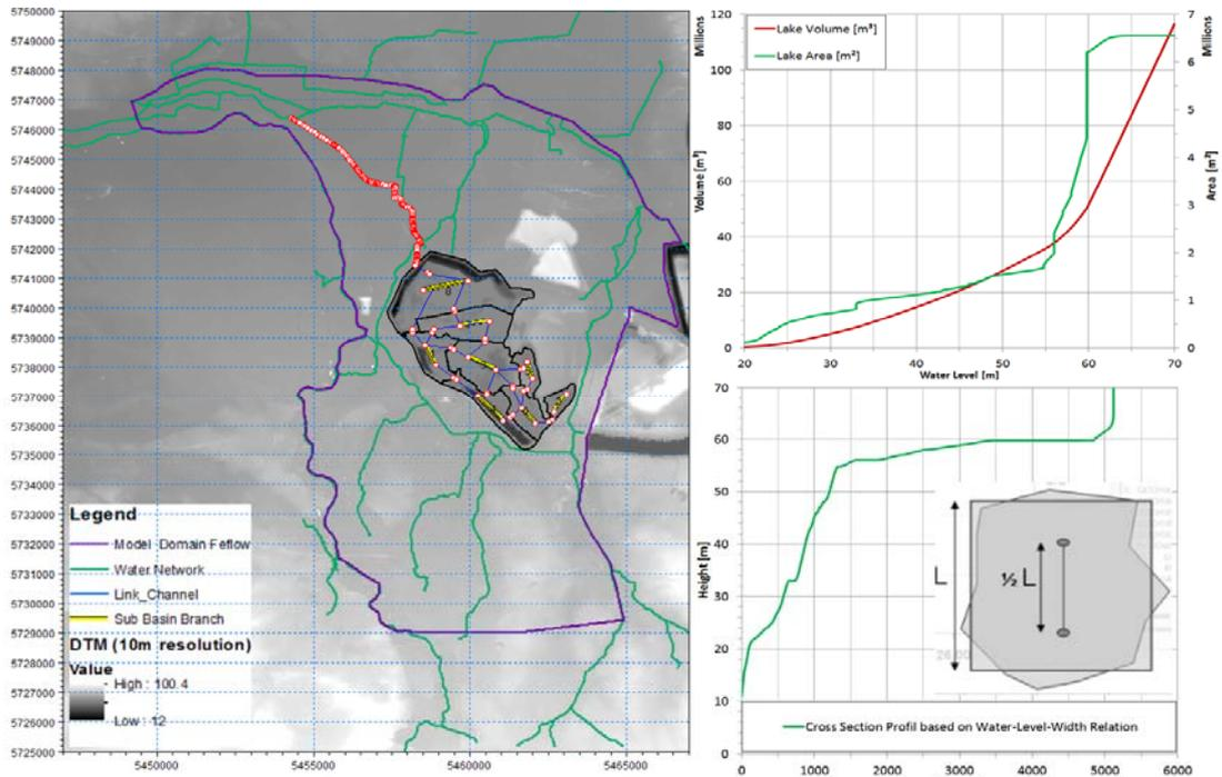
Fig. 3 MIKE11 network and exemplary cross section based on water-level-area relation
