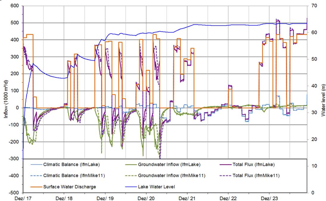
**Fig. 1** Water Level and Flux Components of IfmLake (straight line) and IfmMIKE11 (dashed line)
