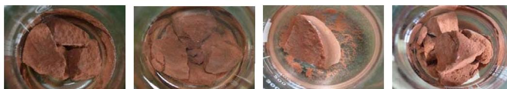
(a) initial in water (b) slight slaking and sand particles flaking (c) slaking and cracks
