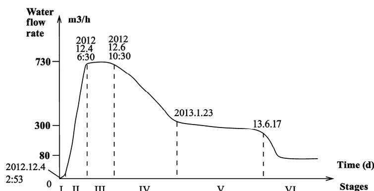
**Fig. 2** Curve of the water inrush flow rate with time
