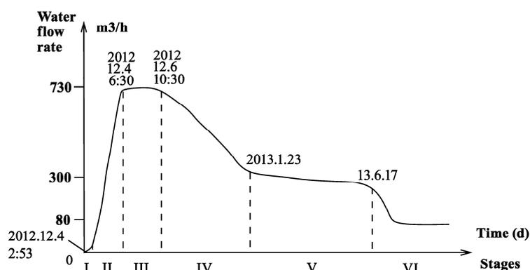
**Fig. 2** Curve of the water inrush flow rate with time
