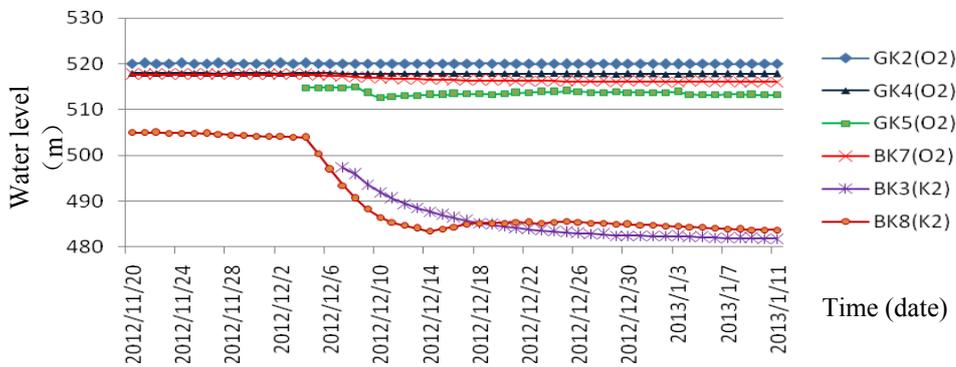
Fig. 3 Curve of the water level with time in the observation boreholes.
