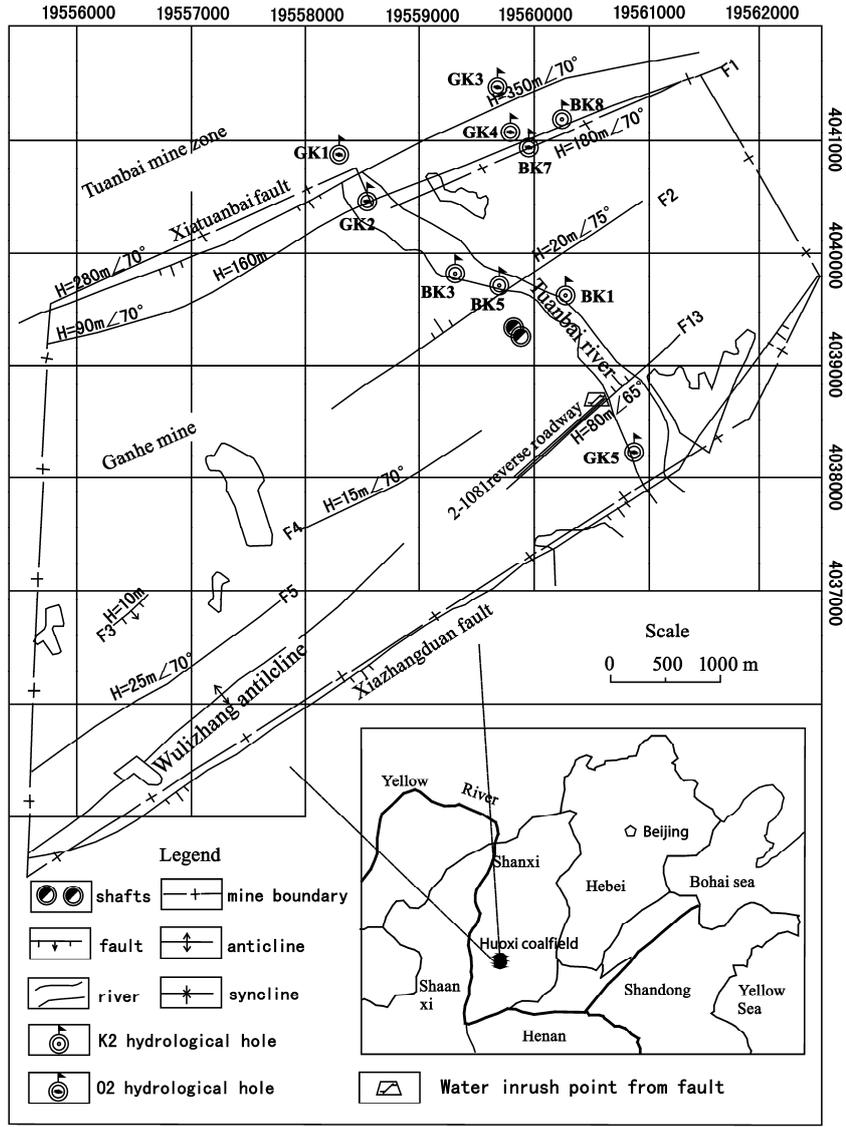
Fig. 1 Structures of the observation boreholes in the Ganhe coal mine.
