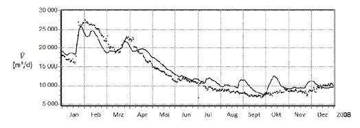
Fig. 3 Course of the discharge rate from the Dickenberg-gallery (line – calculated, dotted – measured) for an area affected by mine water  $A_{mw} = 30$  ha in 2008
