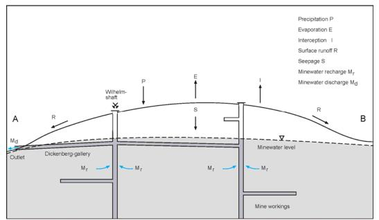
Fig. 2 Schematic sketch of the water movement in the abandoned coal mining area West-Field (position of cross section AB is shown in fig. 1)
