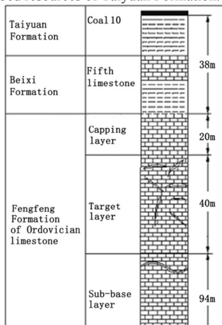
*Fig. 2 Schematic section of Fengfeng formation*
