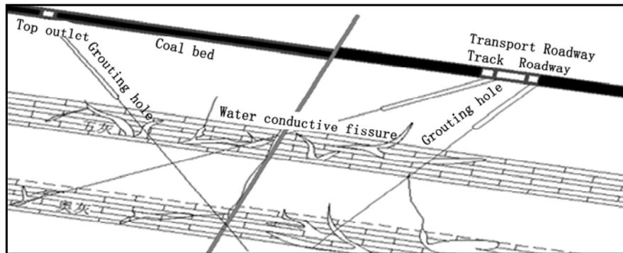
*Fig. 3 Diagrammatic profile of grouting reconstruction*
