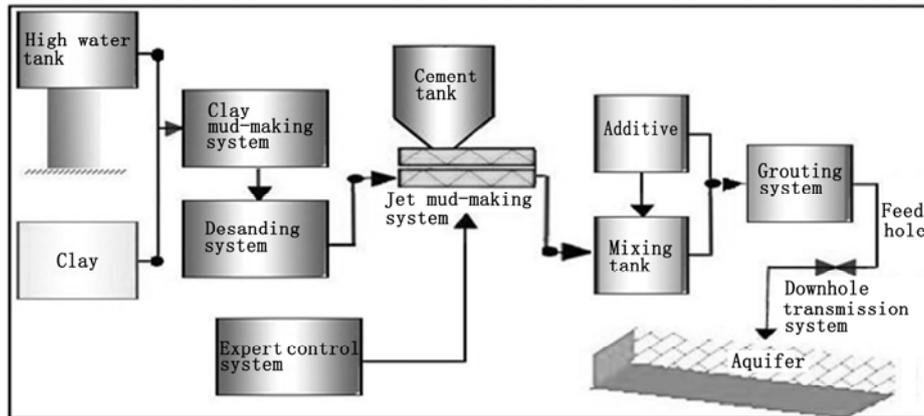
Fig. 4 Process flow chart of grouting reconstruction
