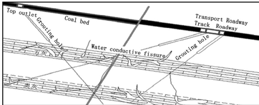
**Fig. 3** Diagrammatic profile of grouting reconstruction
