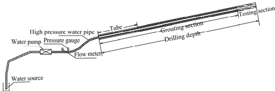
**Fig.3** Diagrammatic drawing of the installation for devices of pressing water in holes
