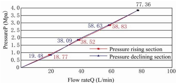
**Fig.4** Curve chart of flow rate and pressure for high pressure pressure water test
