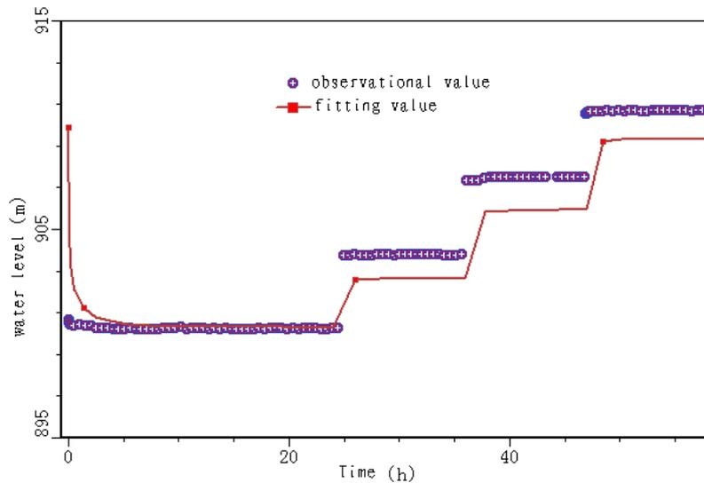
*Fig.4 Pumping test water table fitting of 2# hydrology borehole*
