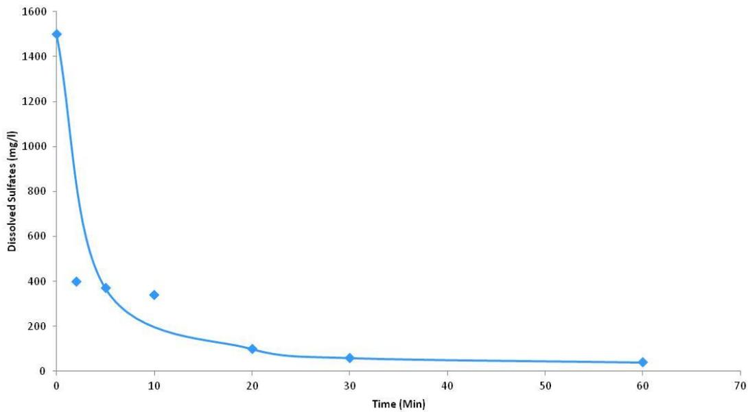
**Figure 5** Sulfate Precipitations Kinetics as Calcium Sulfoaluminate Mineral
