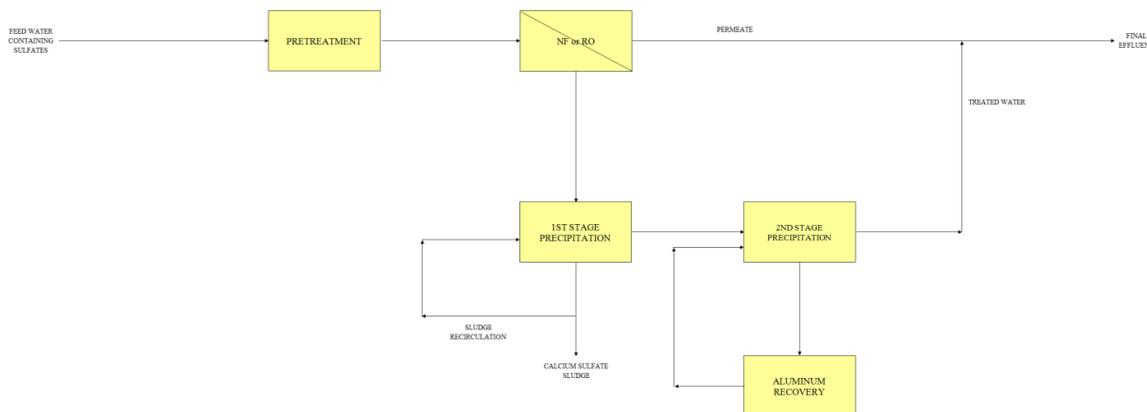
Figure 1 Pilot Flow Diagram
