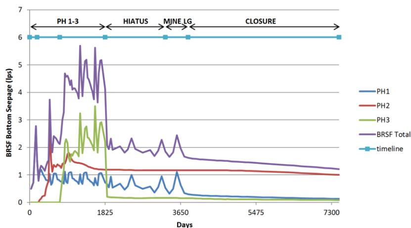
Figure 6 Predicted BRSF seepage flows vs. time
