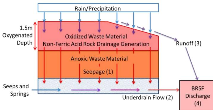
Figure 8 BRSF geochemical conceptual model
