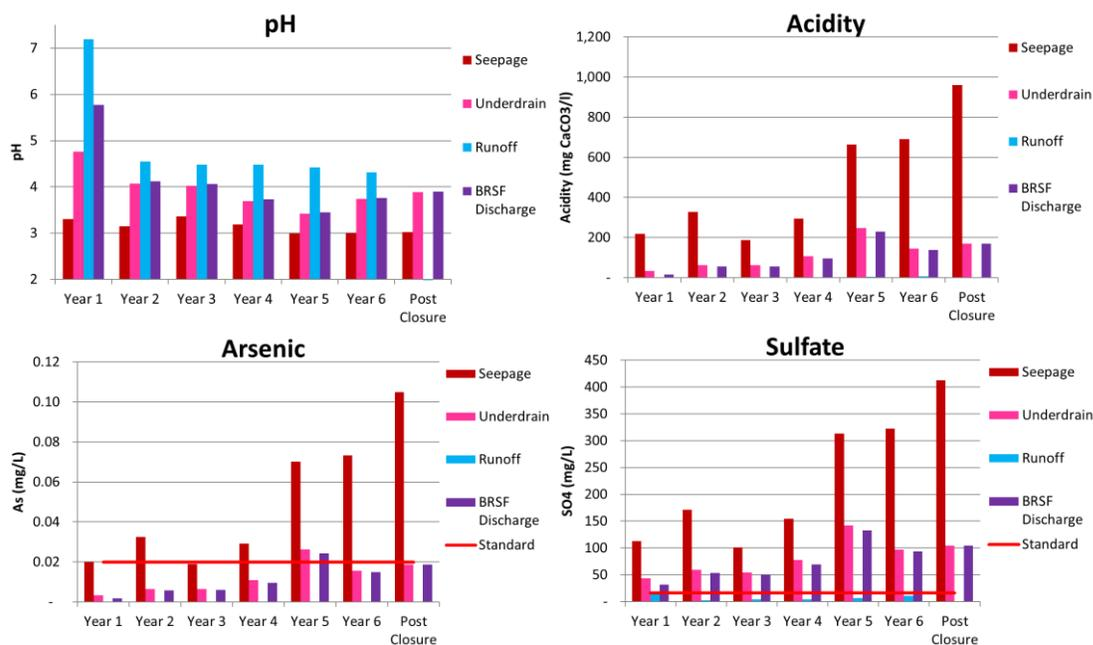
Figure 9 BRSF discharge water quality predictions
