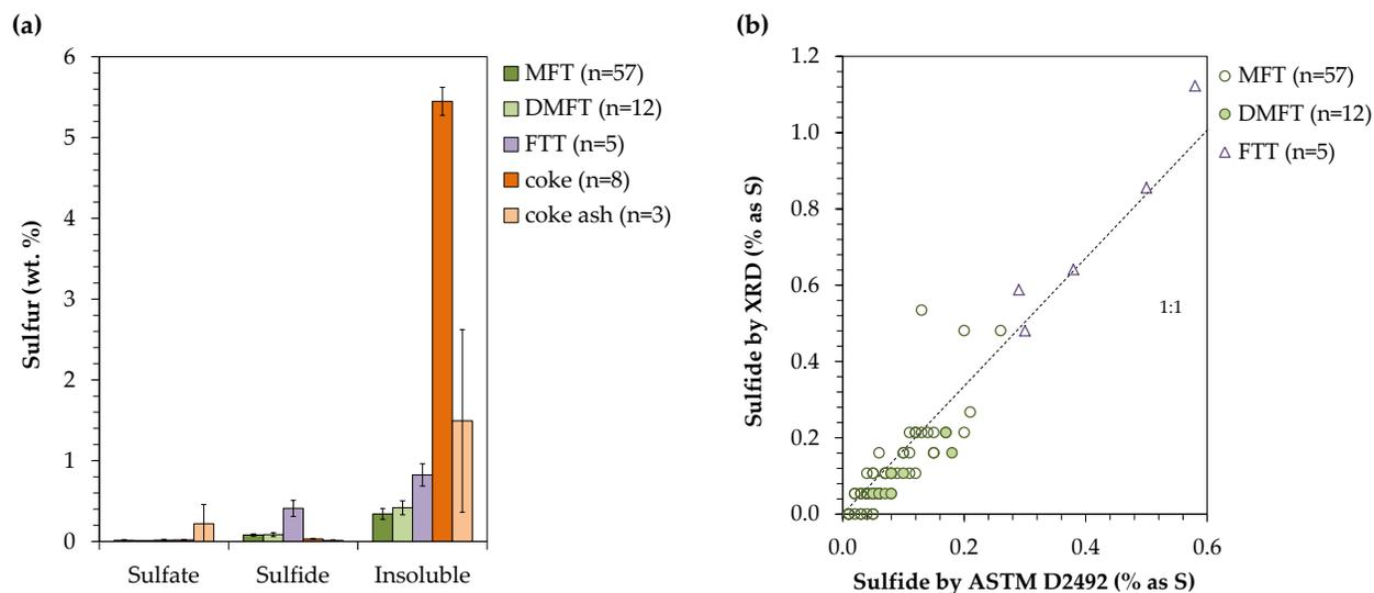
**Figure 1** (a) Sulfur speciation (ASTM D2492) of oil sand tailings, coke, and coke ash presented as arithmetic average values with error bars indicating 95 % confidence intervals; and (b) comparison of sulfide concentrations in tailings as determined by ASTM D2492 and quantitative XRD
