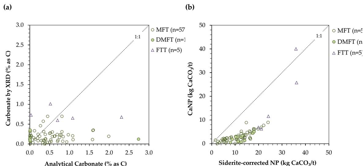
**Figure 2** (a) Comparison of analytical carbonate determined as the difference between total carbon and total organic carbon, and carbonate by quantitative XRD; and (b) comparison of siderite-corrected NP and carbonate NP, whereby CaNP is calculated from calcium and magnesium-bearing carbonates
