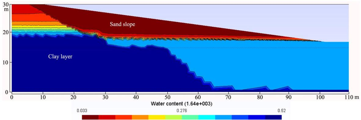
**Figure 6** Water content simulation results without input of precipitation on June 30<sup>th</sup>, 2004
