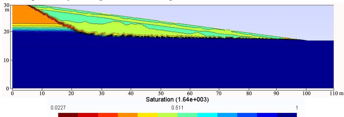
**Figure 8** Simulation of water saturation distribution with input of precipitation on June 30<sup>th</sup>, 2004
