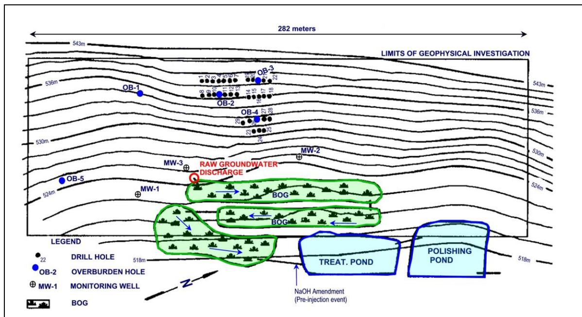
Figure 1 Injection site layout (After Plocus & Rastogi, 1997)
