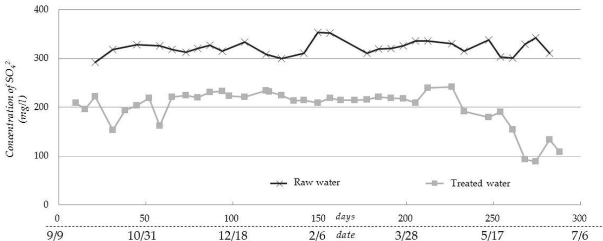
Figure 6 Concentration of sulfate ions in the mine drainage before and after treatment with the anaerobic bioreactor.
