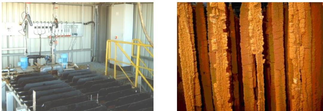
**Figure 1** 1-2.5 m<sup>3</sup>/h pilot plant in Tzschelln (left), where schwertmannite is generated as a byproduct of microbial catalysed lignite mine water treatment on special carrier elements (right)
