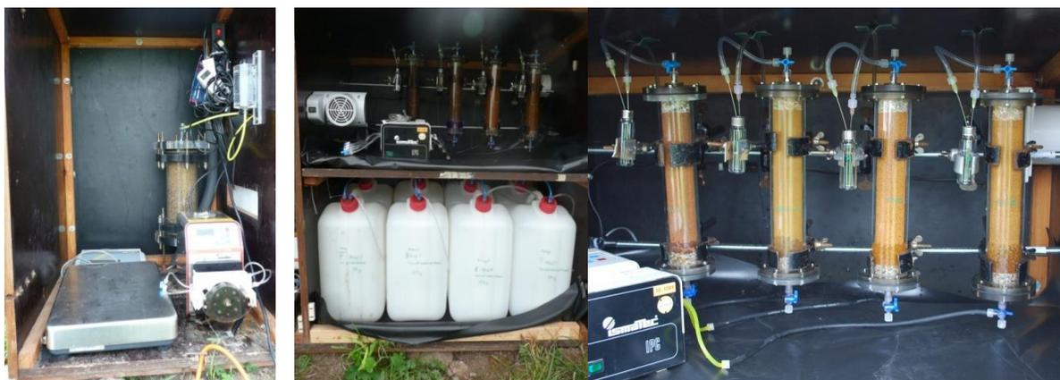
**Figure 4** Field site column test design with a prefilter (sand column) and an admission pressure pump (left), the column test plant with effluent containers (middle) and the Plexiglas columns filled with adsorbents (right)
