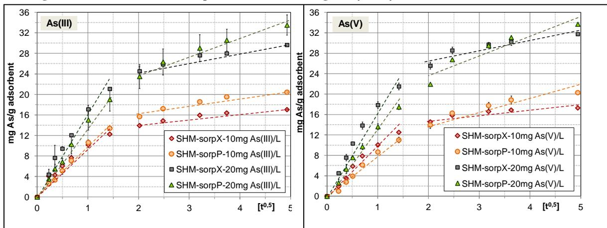
Figure 5 As adsorption kinetics of SHM-adsorbents, 0.5 g ads./L,  $pH_{start}: 7.4 \pm 0.1$ , no pH buffering during the tests
