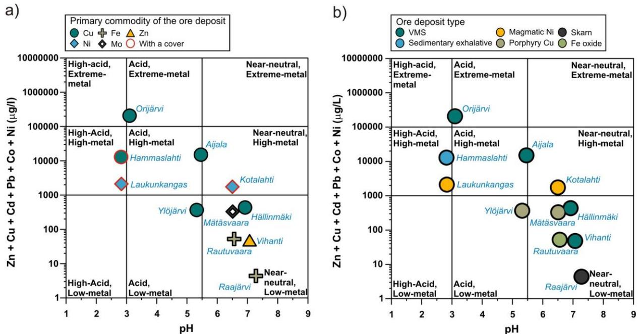
**Figure 2** Ficklin diagrams (Plumlee *et al.*, 1999) of the tailings seepage waters showing the sum of dissolved heavy metals (Zn, Cu, Cd, Pb, Co, Ni) in µg/l plotted against pH value. Mine sites classified a) based on primary commodity of the ore deposit and b) based on genetic type of the ore deposit (VMS = volcanogenic massive sulfide deposit)
