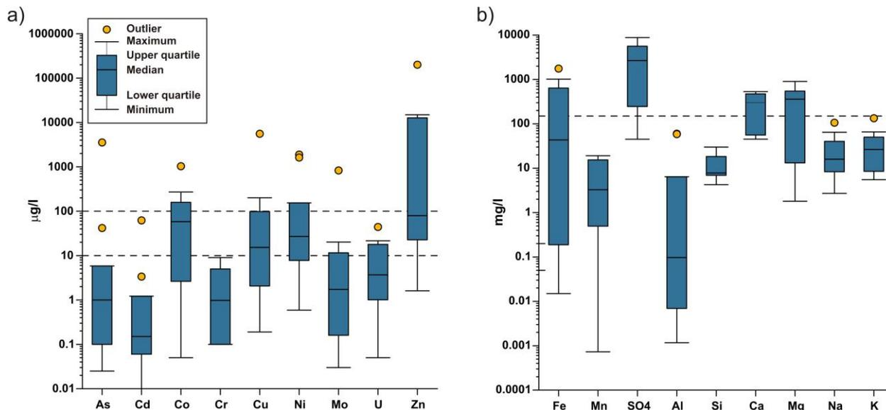
**Figure 3** Box-Whisker plots for selected a) trace metal and b) major element and SO<sub>4</sub> contents of the tailings seepage waters
