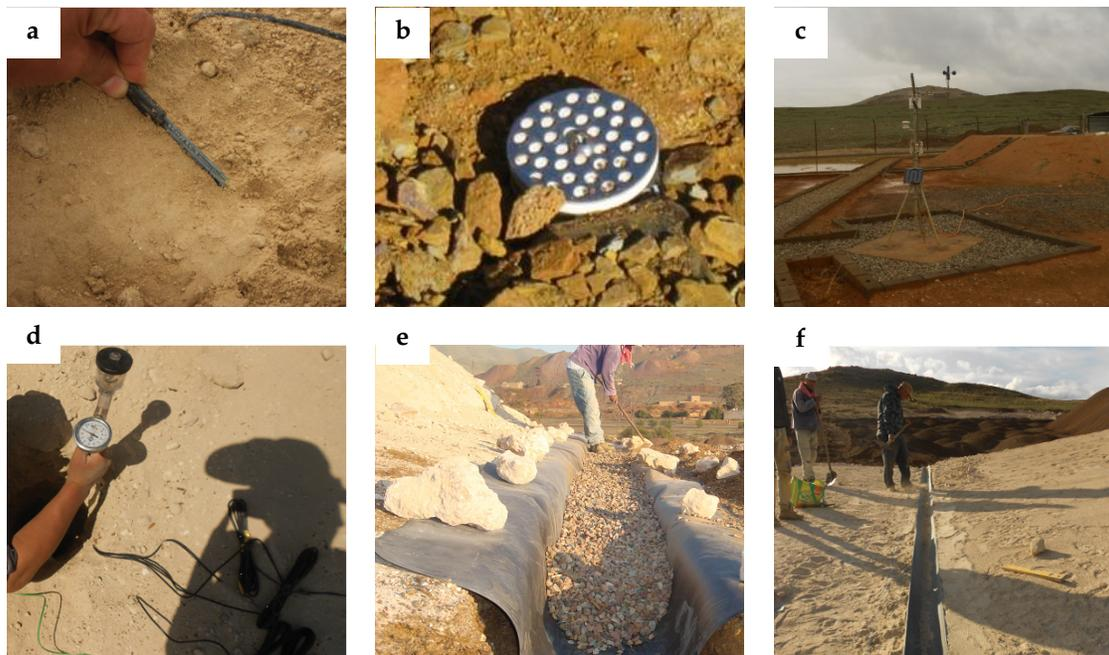
**Figure 3** Photos illustrating the instrumentation used for the monitoring of the inclined SR cover: (a) Volumetric water content sensors (EC5) (b) Matric suction sensors (MPS-2) (c) Weather station (d) JetFill tensiometers (e) Lateral drainage collector (f) Surface drainage collector
