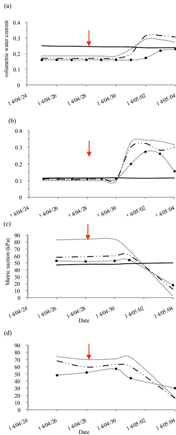
**Figure 4** Measured volumetric water content at depths of 75 cm (a) and 50 cm (b) and measured matric suction at the depth of 75 cm with Watermark (c) and Jetfill (d) stations (the arrow in the figure indicates the wetting event)
