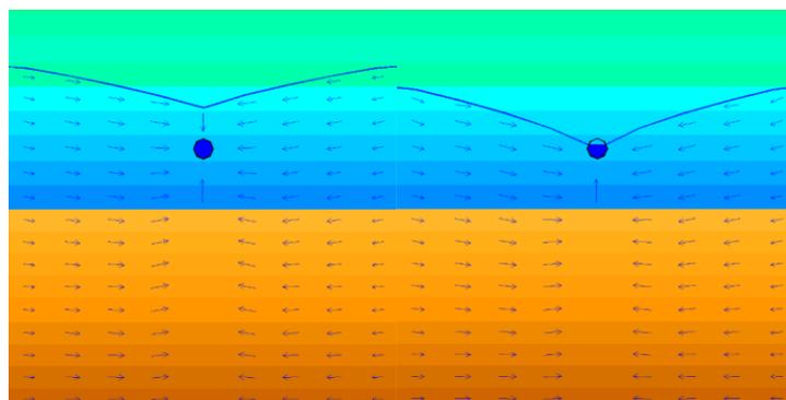
Figure 7 Full (left) and non-full flow (right) to a horizontal well with pressure pipe and open channel flow
