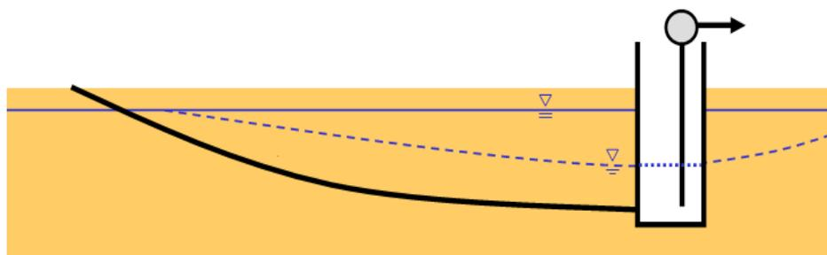
Figure 4 Close-to-surface HDD filter well with collection shaft
