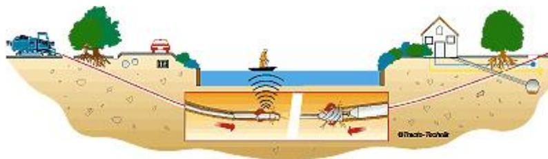
**Figure 1** Schematic presentation of horizontal drilling (Tracto-Technik 2010)
