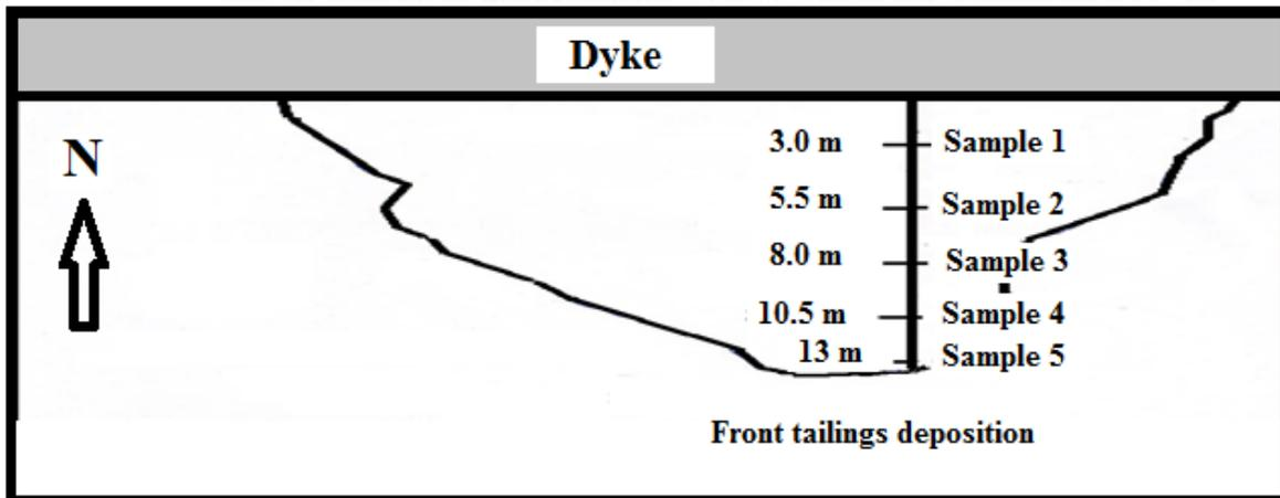
**Figure 2** Samples location during tailings depositions
