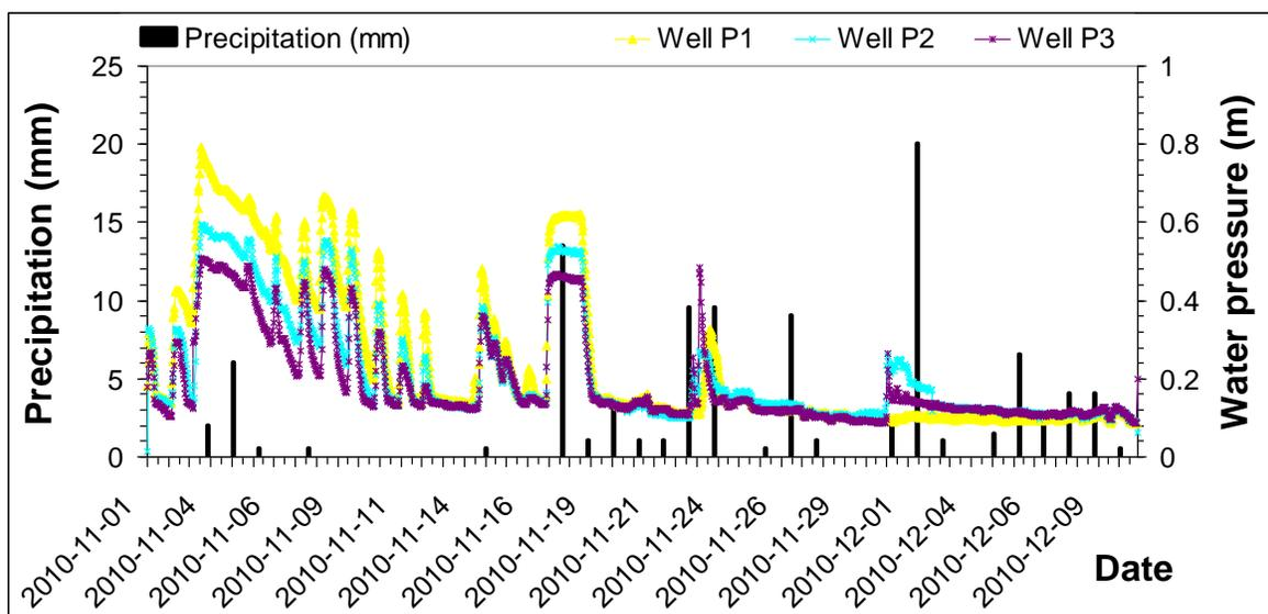
Figure 7 Water pressures measured in the three well points: P1, P2 et P3
