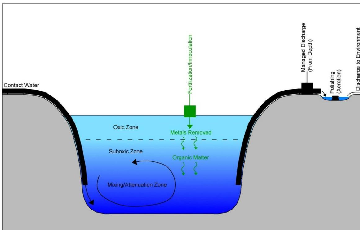
**Figure 4.** Conceptual model that describes a contact water injection system to pit bottom waters and associated removal in support of engineered Se removal system. Fertilization and polishing components
