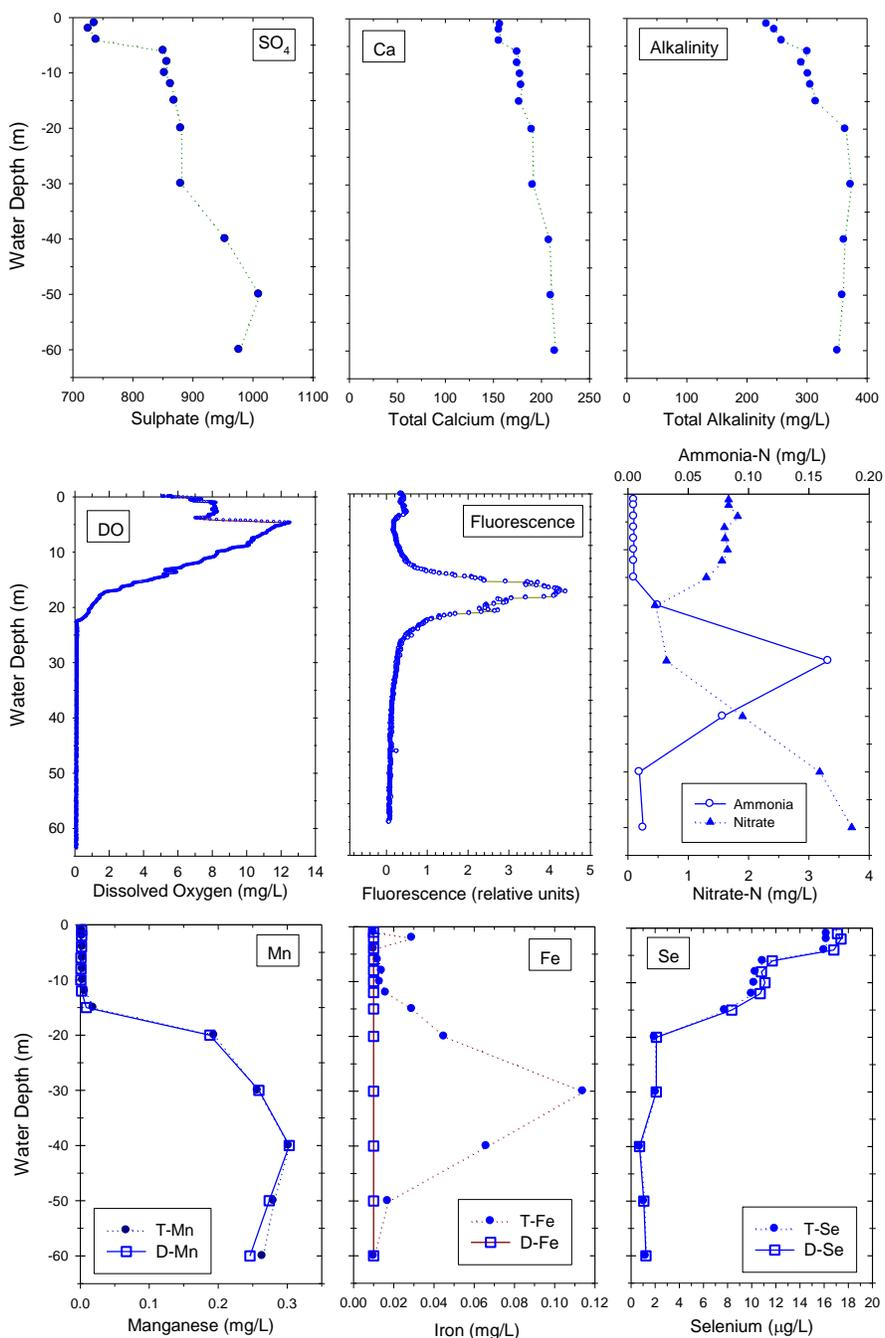
**Figure 2** Vertical profiles of sulfate, total calcium, total alkalinity, dissolved oxygen, fluorescence, nitrate-N, ammonia-N, manganese, iron and selenium in the flooded pit. Data for fluorescence and dissolved oxygen were collected via high vertical resolution *in situ* profiling.
