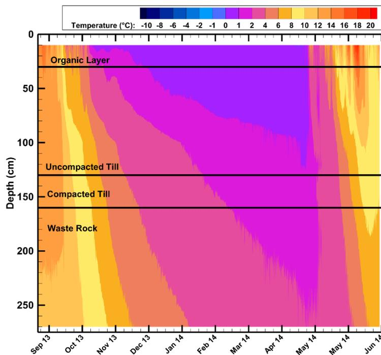
Figure 6 In situ temperature measured within the cover system and waste rock profile of cover system field trial #2.
