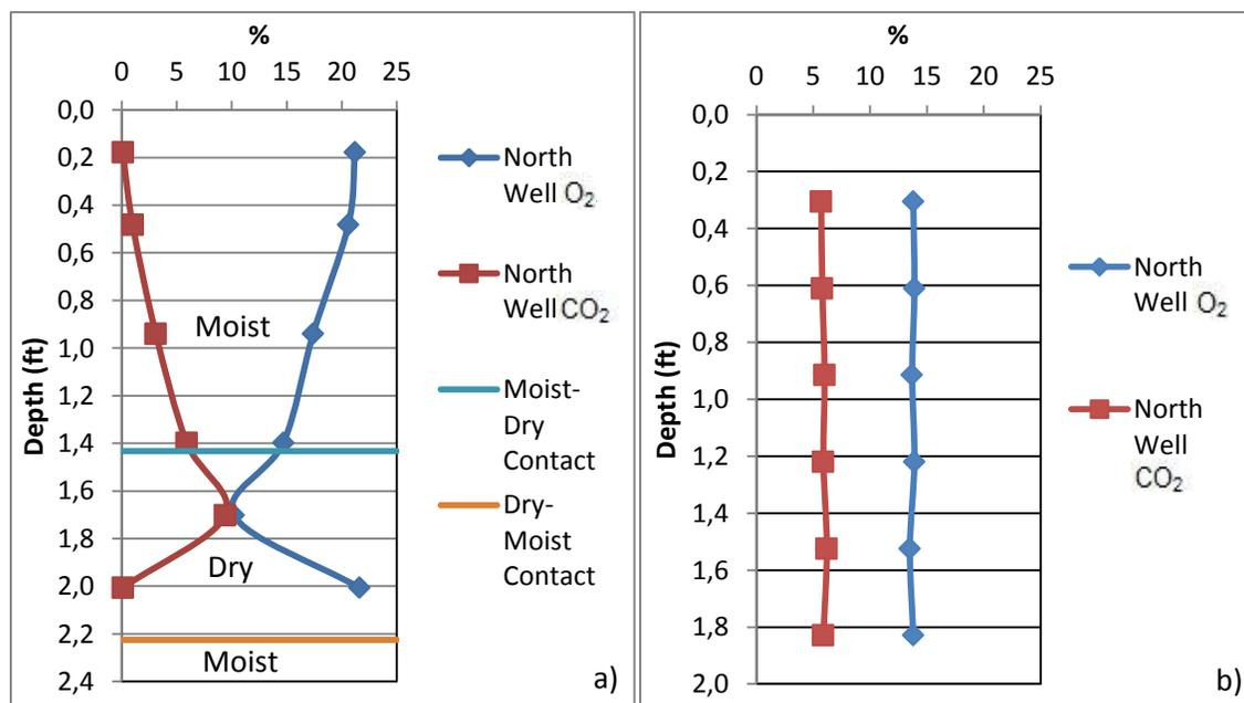
Figure 3 Oxygen (O<sub>2</sub>) and Carbon Dioxide (CO<sub>2</sub>) Profiles: a) Field Leach Pad 1 b) and Field Leach Pad 2
