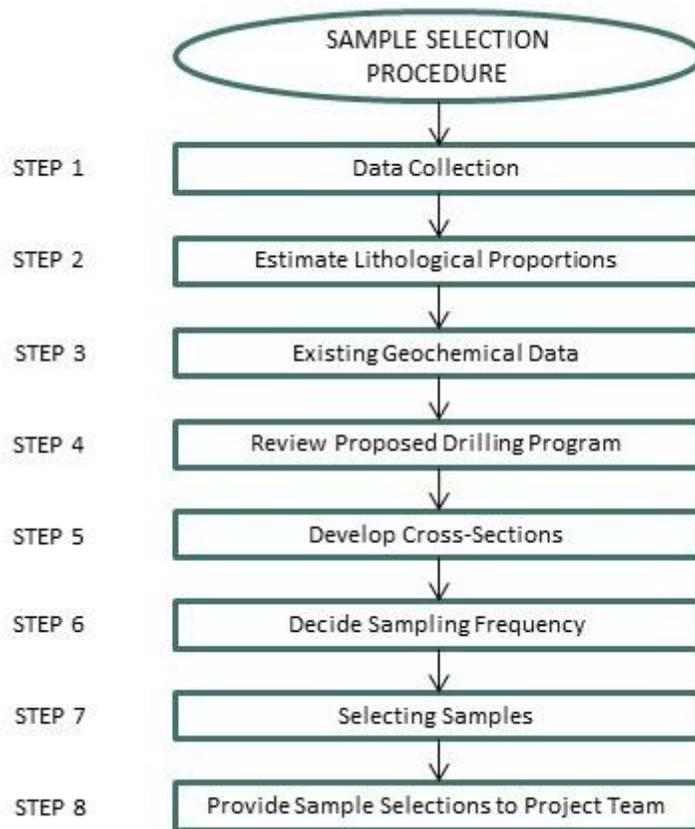
**Figure 2** Sample selection procedure flowchart
