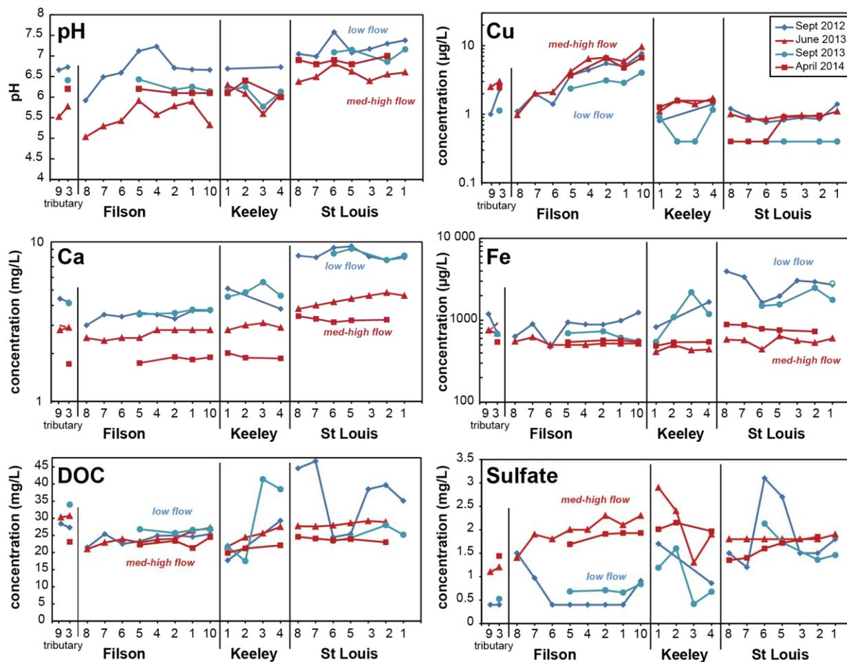
**Figure 3** The pH and dissolved (< 45 µm) concentrations of Cu, Ca, Fe, DOC, and sulfate for each watershed plotted upstream to downstream (right to left for each watershed). Site numbers are given on the x-axis.
