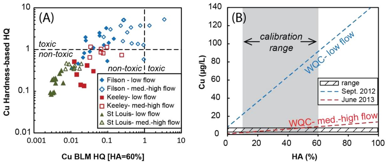
**Figure 6** (A) Hardness-based and BLM-based HQs of chronic Cu toxicity. (B) Range in Cu concentrations and BLM- based chronic WQC for various proportions of HA for low and medium-high flows for Filson Creek site 2.
