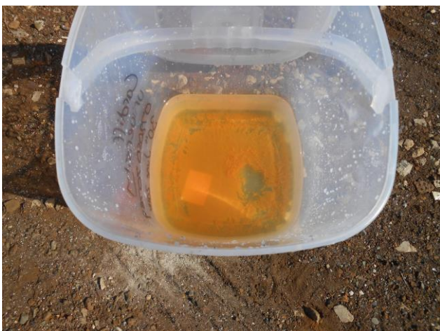
Figure 4 Precipitate formed from mixture of mine water with seawater can clearly be seen at the bottom of the reaction vessel.
