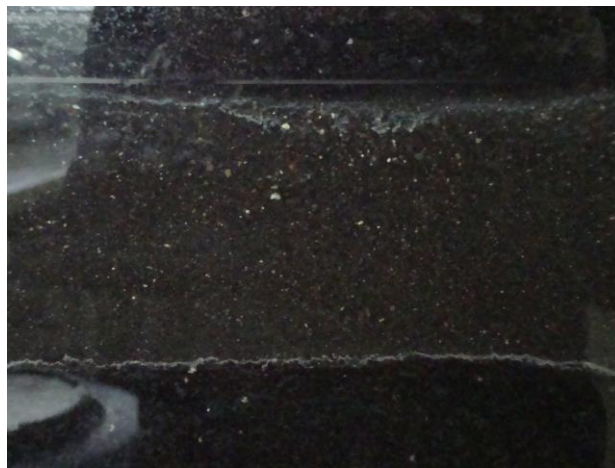
Figure 4 Location of precipitates along layer boundaries. The darker is the organic layer
