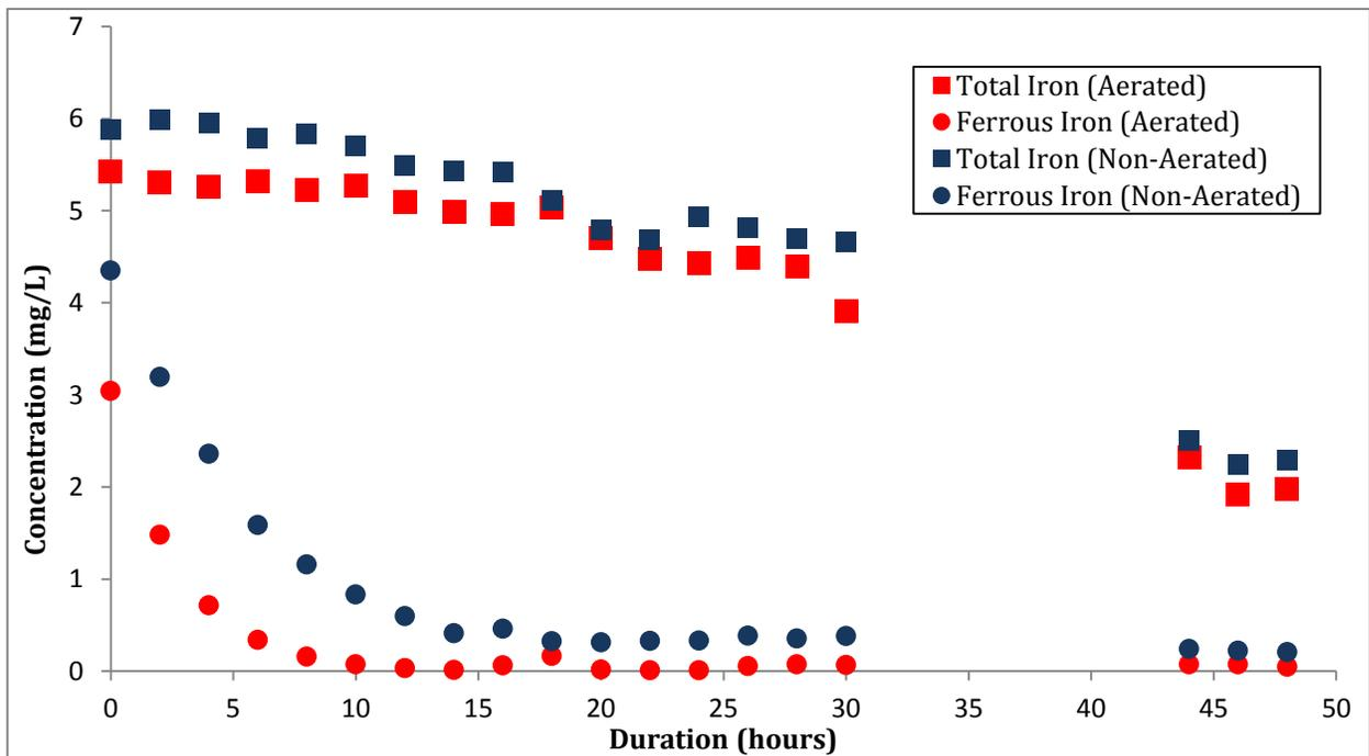
**Figure 4** Change in Fe(II) and total Fe concentration with time in column at Taff Merthyr. Mean pH and initial DO during test = 7.09 and 8.52 mg/L respectively for aerated and 7.11 and 2.62 mg/L for non-aerated
