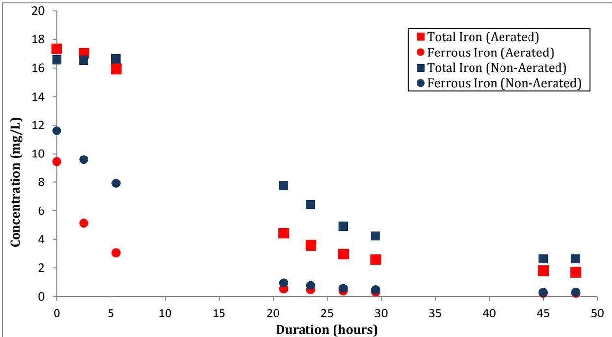
**Figure 2** Change in Fe(II) and total Fe concentration with time in column at Lindsay. Mean pH and initial DO during test = 6.58 and 8.00 mg/L respectively for aerated and 6.59 and 2.67 mg/L for non-aerated
