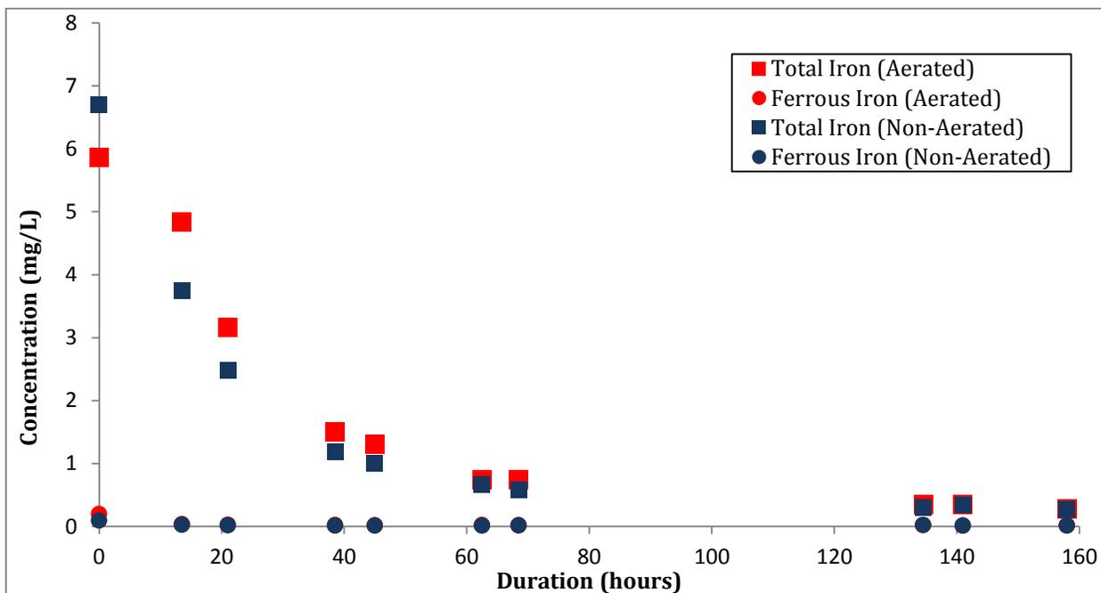
**Figure 5** Change in Fe(II) and total Fe concentration with time in column at active mine site in New Zealand. Mean pH during test = 6.48 for aerated and 6.48 for non-aerated
