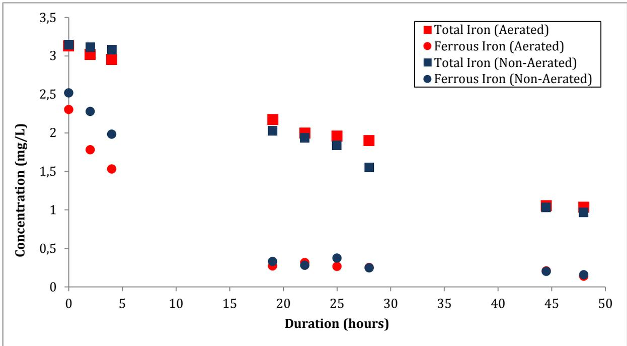
**Figure 1** Change in Fe(II) and total Fe concentration with time in column at Glyncorrwg. Mean pH and initial DO during test = 6.52 and 4.99 mg/L respectively for aerated and 6.17 and 3.44 mg/L for non-aerated
