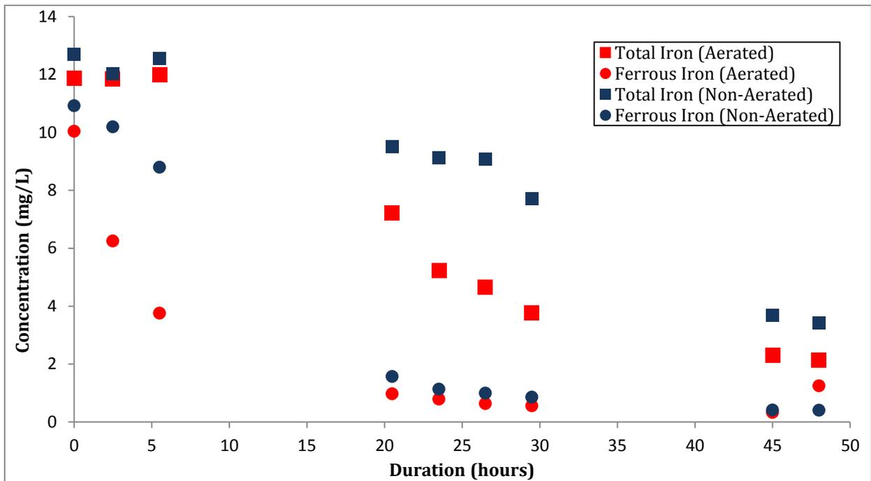
**Figure 3** Change in Fe(II) and total Fe concentration with time in column at Morlais. Mean pH and initial DO during test = 6.06 and 5.01 mg/L respectively for aerated and 6.36 and 3.23 mg/L for non-aerated
