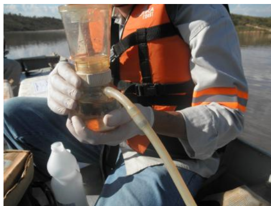
Figure 1 Photo of the water sampling and filtering procedure in the Aroeira tailing dam.
