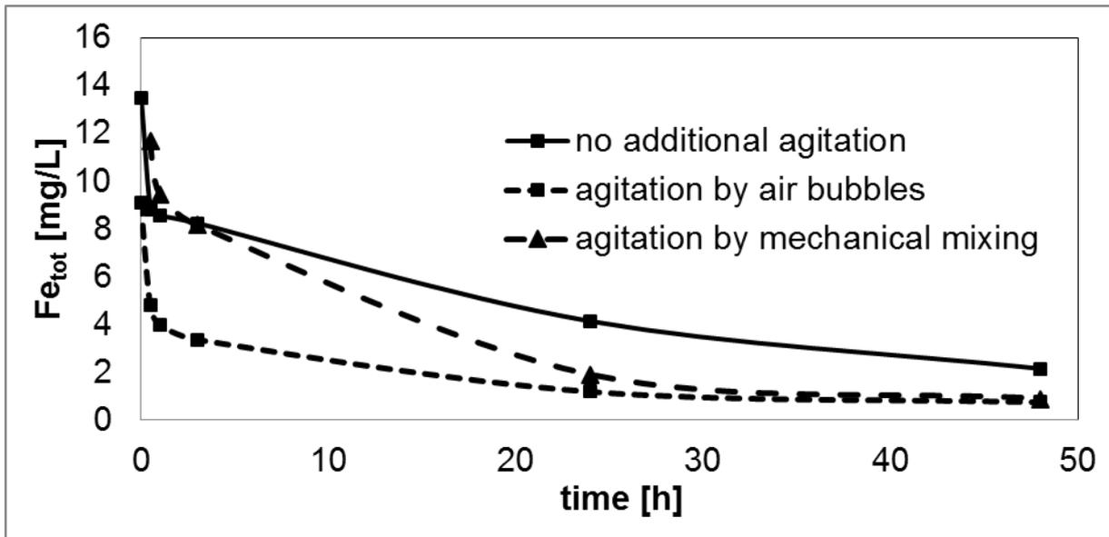
**Figure 5** Investigation of different ways of energy input. Change of total iron concentration with time.
