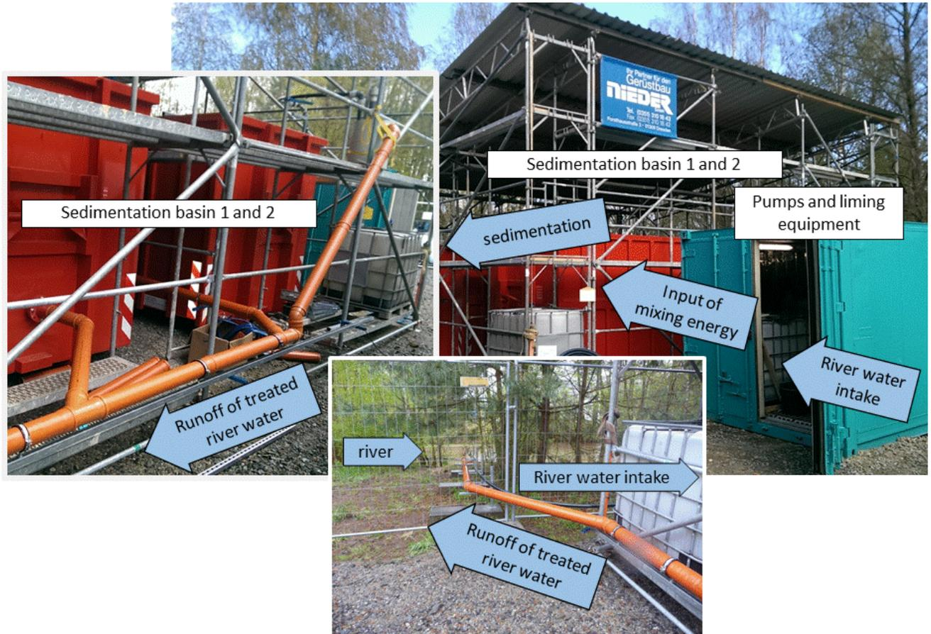
Figure 2 Pilot plant in the field to test various combinations of mixing, liming and sludge recycling.
