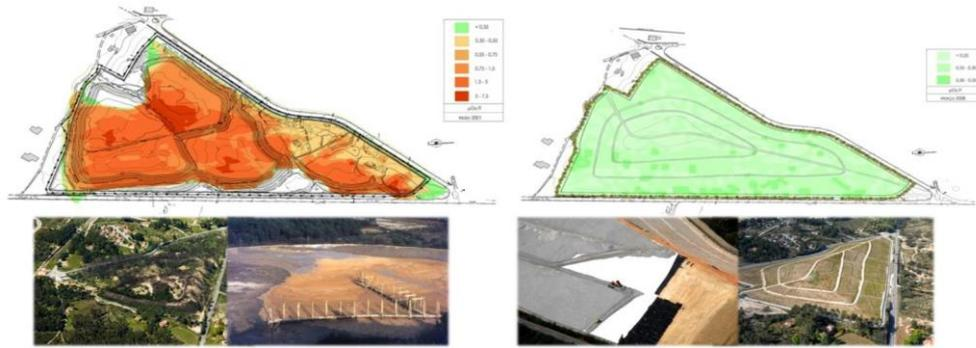
**Figure 3** External radiation results in Old Tailings Dam at Urgeiriça old mining area before and after the remediation works.
