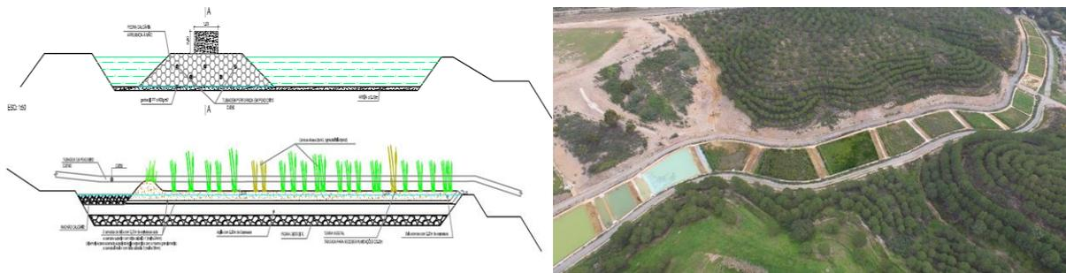
**Figure 10** Lousal passive treatment process with alkaline
