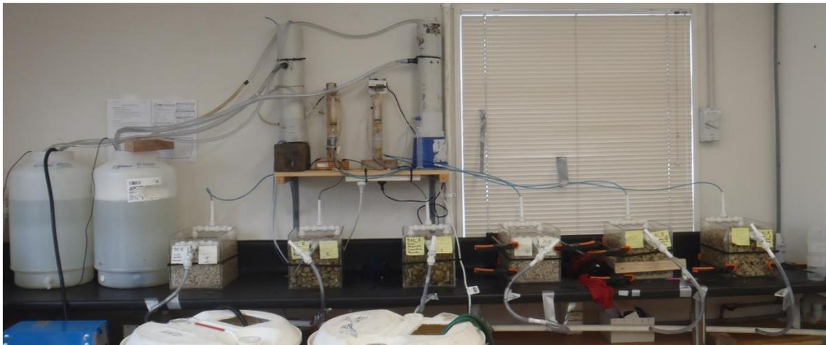
**Figure 1** Experimental set up. The reactors contain: A1. Quartz, A2. Limestone, A3. Limestone and pyrolusite, B1. Quartz, B2. Limestone, B3. Limestone and pyrolusite. Reactors 1-3 receive AMD, and reactors 4-6 receive bactericide treated AMD (B-AMD).
