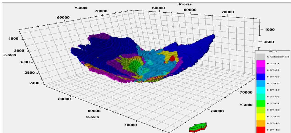
*Figure 1 3D representation of a pit shell defined by geochemical kinetic tests*
