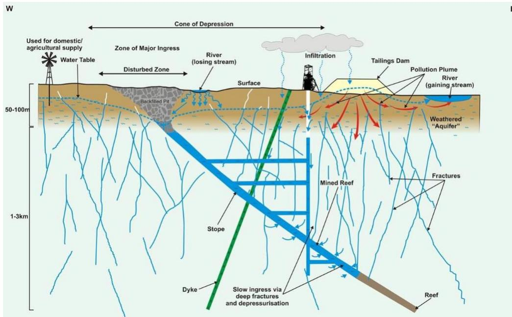
**Figure 1** Hydrogeological model showing flooding mechanisms (taken from: DWA, 2013).
